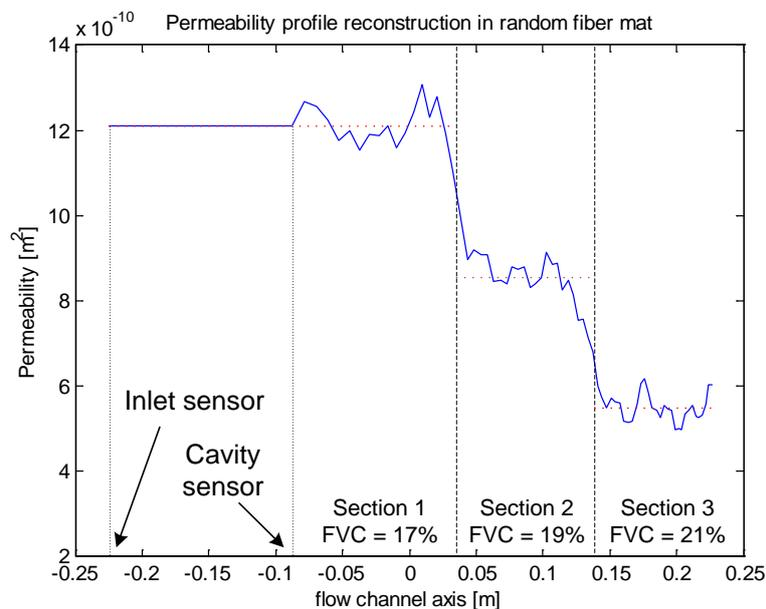
**Figure 1:** Permeability reconstruction during the impregnation of a random fiber mat preform with three FVC sections.
